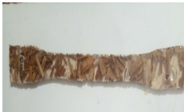
Figure 10: Tensile Test Specimen of 10 Mm Length Fiber Before Testing.
