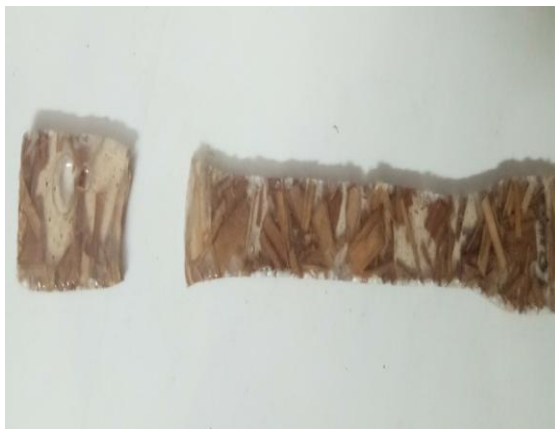
Figure 11: Tensile Test Specimen of 10 Mm Length Fiber After Testing.
